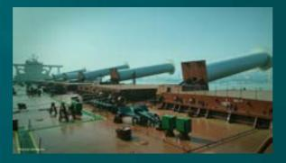
Going under bridges or need space for loading operations? The Norsepower Tilting Foundation<sup>™</sup> is available as an option. Other options include EX proof design and ice prevention.
